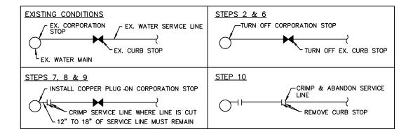
THE FOLLOWING SHALL BE THE MINIMUM NUMBER OF STEPS TAKEN TO ABANDON AN EXISTING WATER SERVICE. THE CONTRACTOR SHALL TAKE ANY AND ALL ADDITIONAL STEPS NECCESARY TO ENSURE WORKER AND PUBLIC SAFETY AND TO RETAIN THE INTEGRIITY OF THE EXISTING WATER MAIN AND ANY AND ALL ADDITIONAL UNDERGROUND UTILITIES THAT MAY BE ENCOUNTERED.ALL WORK SHALL BE PERFORMED IN ACCORDANCE WITH ALL APPLICABLE CURRENT STANDARDS, RULES AND REGULATIONS PUT FORTH BY ALL THE APPLICABLE GOVERMENTAL AGENCIES AND ENTITIES.
