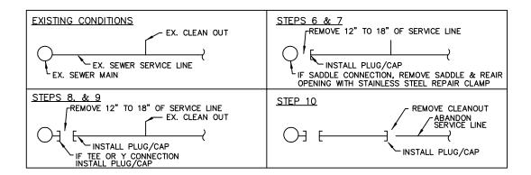
THE FOLLOWING SHALL BE THE MINIMUM NUMBER OF STEPS TAKEN TO ABANDON AN EXISTING SANITARY SERVICE. THE CONTRACTOR SHALL TAKE ANY AND ALL ADDITIONAL STEPS NECCESARY TO ENSURE WORKER AND PUBLIC SAFETY AND TO RETAIN THE INTEGRIITY OF THE EXISTING SANITARY MAIN AND ANY AND ALL ADDITIONAL UNDERGROUND UTILITIES THAT MAY BE ENCOUNTERED. ALL WORK SHALL BE PERFORMED IN ACCORDANCE WITH ALL APPLICABLE CURRENT STANDARDS, RULES AND REGULATIONS PUT FORTH BY ALL THE APPLICABLE GOVERMENTAL AGENCIES AND ENTITIES.
