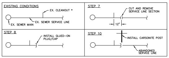
\* - IF A CLEANOUT DOES NOT EXIST, ONE MUST BE INSTALLED IN ACCORDANCE WITH THE L.T.M.U.A. STANDARDS.
