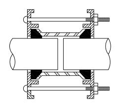
JCM 210 OR 212 DUCTILE IRON COUPLING OR APPROVED EQUAL
