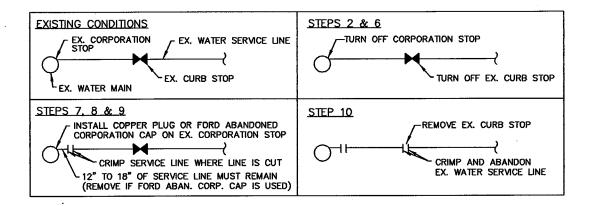
THE FOLLOWING SHALL BE THE MINIMUM NUMBER OF STEPS TAKEN TO ABANDON AN EXISTING WATER SERVICE. THE CONTRACTOR SHALL TAKE ANY AND ALL ADDITIONAL STEPS NECCESARY TO ENSURE WORKER AND PUBLIC SAFETY AND TO RETAIN THE INTEGRITY OF THE EXISTING WATER MAIN AND ANY AND ALL ADDITIONAL UNDERGROUND UTILITIES THAT MAY BE ENCOUNTERED. ALL WORK SHALL BE PERFORMED IN ACCORDANCE WITH ALL APPLICABLE CURRENT STANDARDS, RULES AND REGULATIONS PUT FORTH BY ALL THE APPLICABLE GOVERNENTAL AGENCIES AND ENTITIES.
